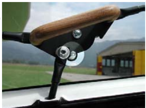
Correct - door secured
