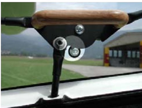
Incorrect - door not secured
