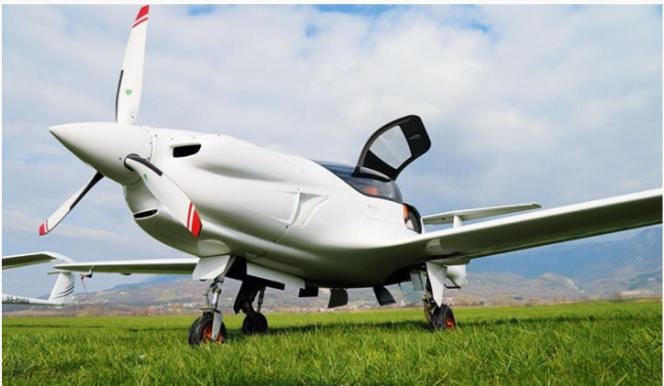
*While it's being tested at an airport with just a grass-strip, the Panthera is a transportation airplane. That said, the beefy trailing link gear doesn't complain about the bumps much.*
