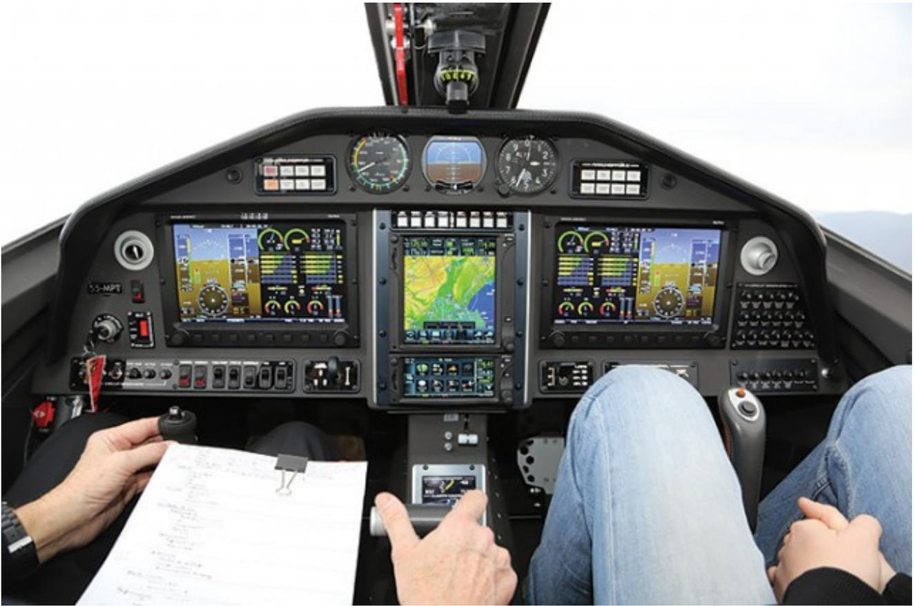
While not the production configuration, the panel in the prototype is superb, easy on the eyes, symmetrical and functional, with two large Dynon Skyview screens and a central column consisting of a Garmin 750 multifunction navigator and a Garmin 635 for communications, both being touch-screen devices. A further addition is promised for the final version, but Pipistrel has sworn everyone to secrecy on the subject.
